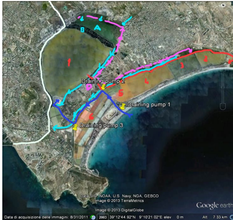
Figure 1: The flows of salt and fresh waters. White line: the main canal from the Mediterranean sea; Salt waters: purple line: from the sea to the first evaporation pond ("Molentargius"). Red line: from the pond to stages of evaporation and to the settling tanks 2-6; fresh waters: pink line: from the purification plant D to the artificial lake A ("Bellarosa minore") and to the other artificial lakes; blue lines: from the artificial lakes to the main canal (white line); B: filterer ecosystem. Blue arrow: creek outflows in basin A. Sources: Google Earth; Mori 1950; www.parcomolentargius.it ; www.apmolentargius.it .
