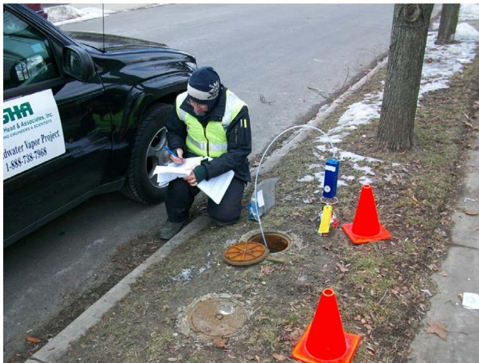
Figure 4: An expert measuring groundwater vapors in Endicott's TCE plume. Photo by author
